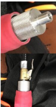
Thanks to this adapter and using a pump or a compressor, inflate the vest to 0,3 bar (5 psi) and check that it does not deflate in less than 5 seconds. (Any pneumatic inflation system, such as those available in filling stations may be suitable for this operation.).
